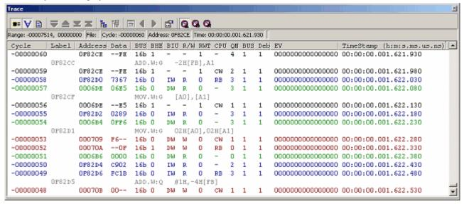
Figure 3.32 Trace window (bus and disassemble mixed display)
